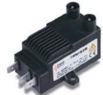
Ignition transformer with capacitive discharge technology for applications in condensing boilers and atmospheric gas burners. Developed to produce more power to the classics on board lighters, filtered against electromagnetic interference and available with output for mono-electrode flame detection.
